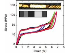
Oligocrystalline shape memory alloys are microstructurally designed shape memory alloy structures in which the total surface area exceeds the total grain boundary area. How the formation of an oligocrystalline grain architecture improves the performance of Cu-based, polycrystalline shape memory alloys to a point where their properties resemble those of single crystals is demonstrated.
