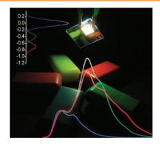
The device operation of a single-layer white-emitting polymer light-emitting diode (PLED) is investigated. From single-carrier devices it is determined that the red and green dyes act as electron traps. Taking into account trap-assisted recombination on the dyes and Langevin recombination on the blue backbone, the color shift of the white-emitting PLEDs can be explained.
