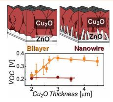
Electrodeposited bilayer and nanowire  $\text{Cu}_2\text{O-ZnO}$  photovoltaics are studied as a function of the  $\text{Cu}_2\text{O}$  absorber thickness, ZnO nanowire length, and nanowire seed layer. The low open-circuit voltage of nanostructured  $\text{Cu}_2\text{O-ZnO}$  cells is shown to result from an incompatibility between the desired nanostructure spacing and the  $\text{Cu}_2\text{O}$  thickness required to form the full built-in bias that inhibits recombination.
